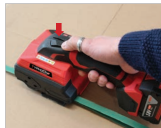
Saldatura e taglio tramite pulsante Welding and cutting by button
